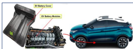
Exhibit 4.1.2: Li-ion battery pack for TML
